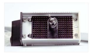
Figure 8-2. Hypertronics plug of 128-channel GSN
