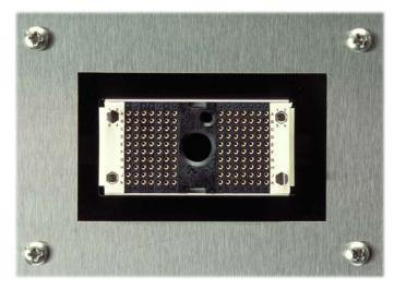
Figure 8-1. Multicontact Hypertronics receptacle (128-channel Net Amps 200 amplifier)
