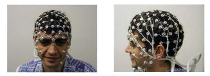
Figure 2-1. 128-channel HCGSN, front (left) and side (right) views
