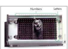
**Figure 9-8.** Note the numbers and letters marked on the connector
