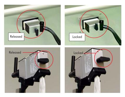
Figure 8-3. Hypertronics plug released (left) and locked (right)
