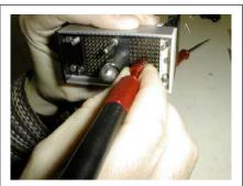
**Figure 9-9.** Remove the contact using the extraction tool
