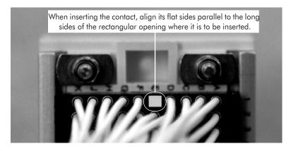
Figure 9-13. View of connector before inserting contact
