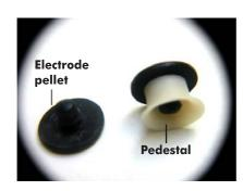
Each electrode pellet is set into the bore of the HydroCel Hydrating Skin Interface Chamber, a soft, plastic pedestal (Figure 2-6).
