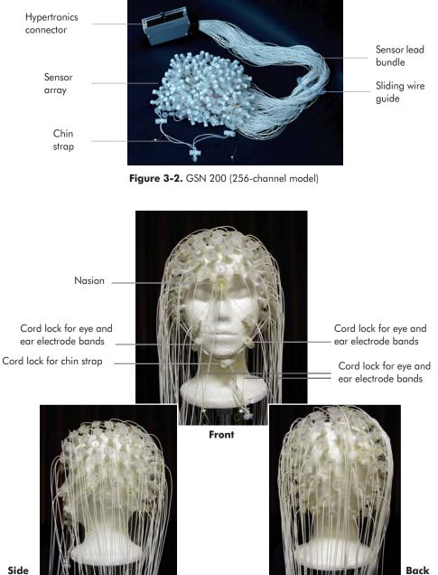
views of the GSN 200. Most of the wire management is done manually, by grouping wires together with plastic stays.
