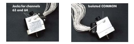
Figure 3-9. Infant Net special Hypertronics connector, with outrider jacks strapped to isolated common
