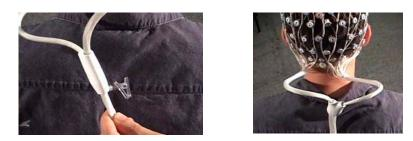
Figure 6-21. Secure the Y clip to the collar
