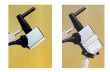
Figure 8-5. Plugging GSN into the GSNIC and the articulated arm
