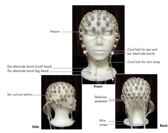
The HCGSN also contains stabilizer pedestals to keep the bottom row of pedestals from overturning, and cut-out sections for the ears. Figure 2-3 shows these features and others in front, side, and back views of the HCGSN.
