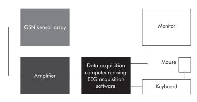
Figure 1-4. Functional block diagram of a typical GES
